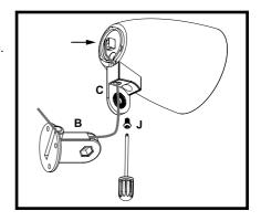
4. Firmly mount the seal cap back to the Speaker.
