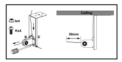
4. Using a screwdriver attach the Mount Arm to the Speaker.
