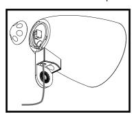
6. Firmly mount the seal cap back to the Speaker.
