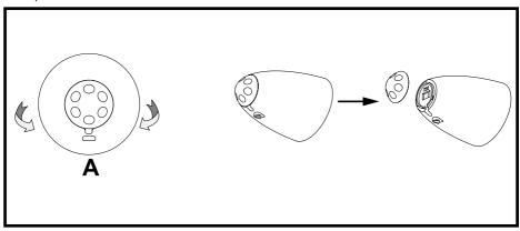
5. Plug in the Quick Speaker Connector – Terminal Block to the terminal socket which is located under the seal cap.
