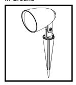
1. Using a mallet pound the Ground Stake into the ground. You can use a wooden block to protect the top part of the Ground Stake.
