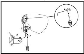
5. Firmly mount the seal cap back to the Speaker.
