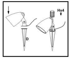
6. Set the required Speaker position and tighten the Hex Socket Head Screw (check "Vertical angle regulation" for more details).
