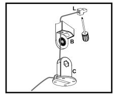
3. Plug in the Quick Speaker Connector – Terminal Block to the terminal socket (check "Connect the sound source" for more details). Using a screwdriver attach the Mount Arm to the Speaker.
