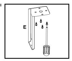
3. Run the speaker cable through the Surface Mount and using a screwdriver attach the Surface Mount firmly to the Ceiling-Wall mount.
