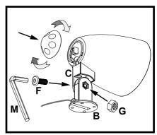
Set the speaker in the down position.Using a screwdriver attach the Surface Mount to the Ground Stake.
