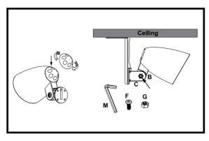
6. Set the required Speaker position and tighten the Hex Socket Head Screw (check "Vertical angle regulation" for more details).
